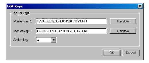
Choose two 112-bit *encryption keys* to use with your network. The quickest way is to generate random keys using built-in function. Note that there are two master keys, but only one of them (usually key *A*) is used at any given time. The second key is a backup. If you find that current key is somehow compromised, you can switch to the backup key and gradually replace the compromised key on smartcards.
