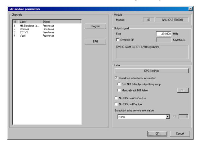
Enter output signal *frequency*. Click on each *program*, correct the *label* (channel name) if needed, and select *conditional access mode* for the program. If you choose to encrypt the channel (*scrambled*), select the logical program number for this channel.
