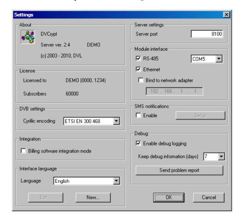
Check *RS-485* and select virtual serial port to which *USB* <-> *RS-485* converter is connected (refer to 3.3 Equipment connection section above). If you're not using any modules with *RS-485* interface, uncheck *RS-485* checkbox.
