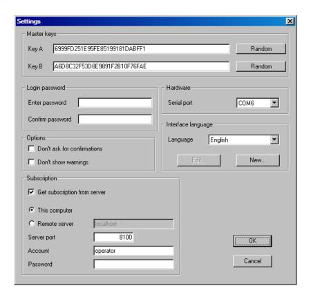
Enter two 112-bit *encryption keys* to use with your network. *Make sure that you correctly copy keys from the server!* Otherwise the smartcards wouldn't decode the channels.
