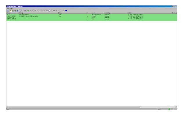
For modules with ASI digital inputs, click on the module and run *input stream selection utility* (select icon from toolbar). Follow the utility prompts to scan input streams and select which TV channels to include in the output stream:
