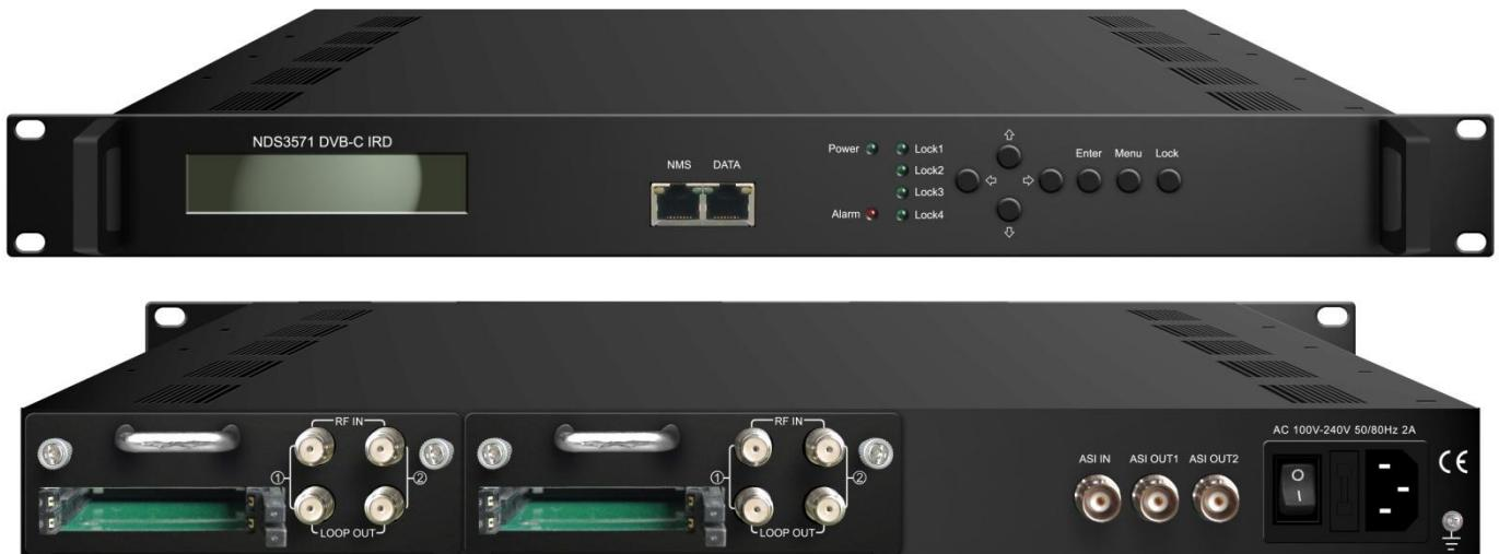
Demodulation Module = 2\*RF/Loop out + 2\*CAM + 2\*Smartcard
